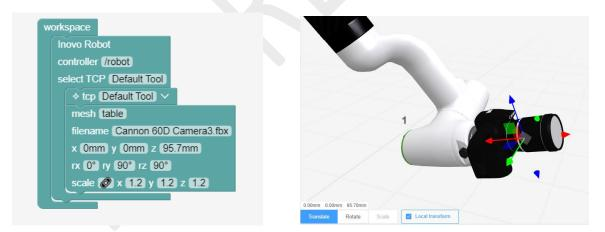
You can also position it by selecting the mesh block in the workspace and then dragging the arrows in the 3D view. Tick the 'Local Transform' check box to move it in the tool frame.
